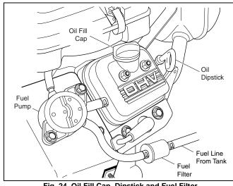
Fig. 24 Oil Fill Cap, Dipstick and Fuel Filter
